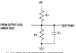
C L INCLUDES JIG AND PROBE TOTAL CAPACITANCE
